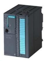
\*\*\*Spare part\*\*\* SIMATIC S7-300, CPU 312C Compact CPU with MPI, 10 DI/6 DQ, 2 high-speed counters (10 kHz) Integr. power supply 24 V DC, Work memory 32 KB, Front connector (1x 40-pole) and Micro Memory Card required
