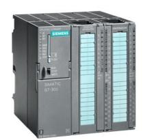
SIMATIC S7-300, CPU 314C-2PN/DP Compact CPU with 192 KB work memory, 24 DI/16 DO, 4 AI, 2 AO, 1 Pt100, 4 high-speed counters (60 kHz), 1st interface MPI/DP 12 Mbit/s, 2nd interface Ethernet PROFINET, with 2-port switch, Integr. power supply 24 V DC, Front connector (2x 40-pole) and Micro Memory Card required
