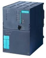
\*\*\*Spare part\*\*\* SIMATIC S7-300 CPU 317-2 PN/DP, Central processing unit with 1 MB work memory, 1st interface MPI/DP 12 Mbit/s, 2nd interface Ethernet PROFINET, Micro Memory Card required
