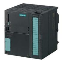
SIMATIC S7-300, CPU 317T-3 PN/DP, Central processing unit for PLC and technology tasks, 1024 KB work memory, 1st interface MPI/DP 12 Mbit/s, 2nd interface DP (drive), 3rd interface Ethernet PROFINET with 2-port switch, Integr. I/O for technology, Front connector (1x 40-pole) and Micro Memory Card min. 8 MB required
