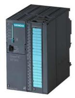
\*\*\*Spare part\*\*\* SIMATIC S7-300, CPU 312C Compact CPU with MPI, 10 DI/6 DQ, 2 high-speed counters (10 kHz) Integr. power supply 24 V DC, Work memory 32 KB, Front connector (1x 40-pole) and Micro Memory Card required
