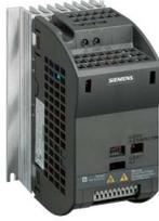
SINAMICS g110 - cpm110 AC-drive filter 1AC200-240v +10/-10% 47- analog input ct 0.37KW vt 0.37K ct-overload 150% 60s 150 x 90 x (hwx) protection IP20 ambient to +50 deg c without bop without rs485-interface Product reached PM410 (product cancelled) on 10/01/19 long delivery time of at least 60 working days. See for replacements: siemens.com/mm4-convert
