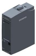
SIMATIC ET 200SP, digital output module, DQ 4x 24..230V AC/2A Standard suitable for BU type B1, Color code CC41, Module diagnostics
