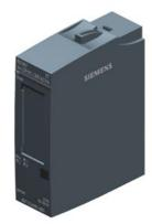
SIMATIC ET 200SP, Relay module, RQ NO 4x 120V DC..230VAC/5A ST. 4 normally open contacts, isolated contacts, packing unit: 1 piece, fits to BU-type B0 and B1, Colour Code CC40, substitute value output, module diagnostics for: supply voltage
