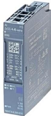
SIMATIC ET 200SP, Analog input module, AI 2 X SG 4-/6-wire High Speed, two-channel analog input module for strain gauges (full bridges), Color code CC00, Module diagnostics 28/16 bit, 2xLC load cell interface (1-4mV/V), suitable for BU type A0, packing quantity: 1 unit
