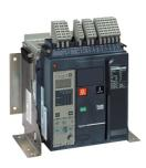
Circuit breaker frame, MasterPact NT10H2, 1000A, 50kA/440VAC 50/60Hz (Icu), 3 poles, fixed, without control unit
