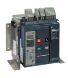
Circuit breaker frame, MasterPact NT08H1, 800A, 42kA/440VAC 50/60Hz (Icu), 3 poles, drawout, without control unit
