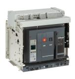
Circuit breaker frame, MasterPact NW16H1, 1600A, 65kA/440VAC 50/60Hz (Icu), 4P, right Neutral, fixed, no control unit
