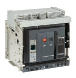
Circuit breaker frame, MasterPact NW32H1, 3200A, 65kA/440VAC 50/60Hz (Icu), 4P, right Neutral, fixed, no control unit
