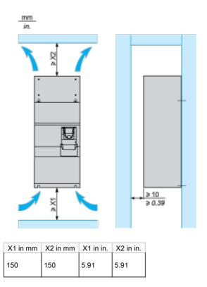
These drives can be mounted side by side, observing the following mounting recommendations:
