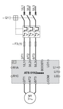
A1: Soft start/soft stop unit(1) For type 2 coordinationQ1: Motor circuit-breakerF3: 3 fast-acting fuses
